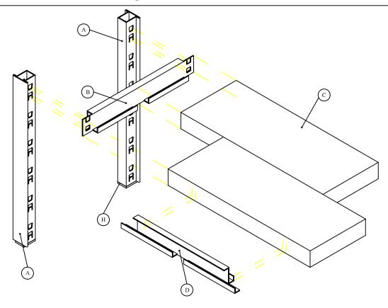
1) Place the uprights (A) in pairs, in a vertical position, making sure the black rubber (H) is on the floor, or that the slots of the uprights are as shown in the design.
